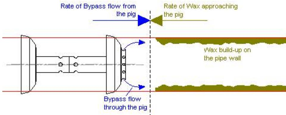
To avoid a wax accumulation ahead of the pig, then the rate of bypass flow from the pig must be greater than the rate of wax approaching the pig.
