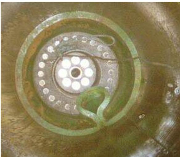
View on large diameter seal which has been allowed to buckle naturally into the small diameter line. This leads to high friction and damage to the seal.
