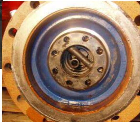
Same disc in 257 mm pipe takes on a cup shape but does not buckle
