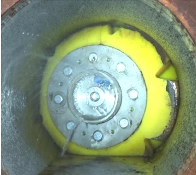
Figure 9 – Still from video of open-ended test showing pig negotiating a bend and leakage through the pig body and bolts. This leakage would be difficult to measure using a flow meter and pig signallers due to errors.
