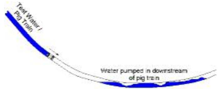
Fig. 4 – Water pumped in ahead of the pig train to dampen motion
