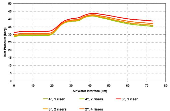
Fig. 7 – Inlet Pressure for different hose diameters and number of risers
