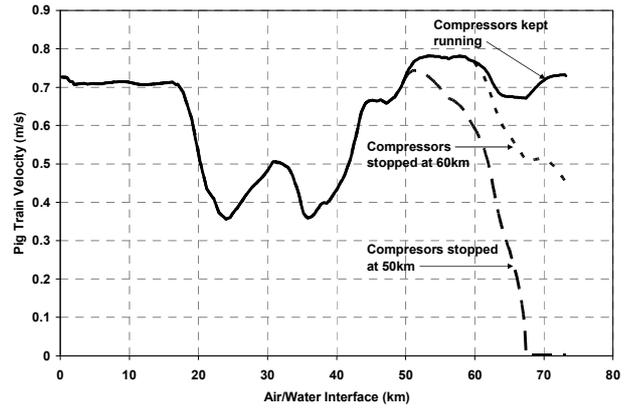
Fig. 9 – Effect of stopping pumping
