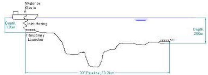
Fig. 1 – Schematic of field layout
