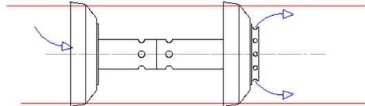
Conversely, an increase in flow rate can mean that there is insufficient percentage bypass through the pig.
